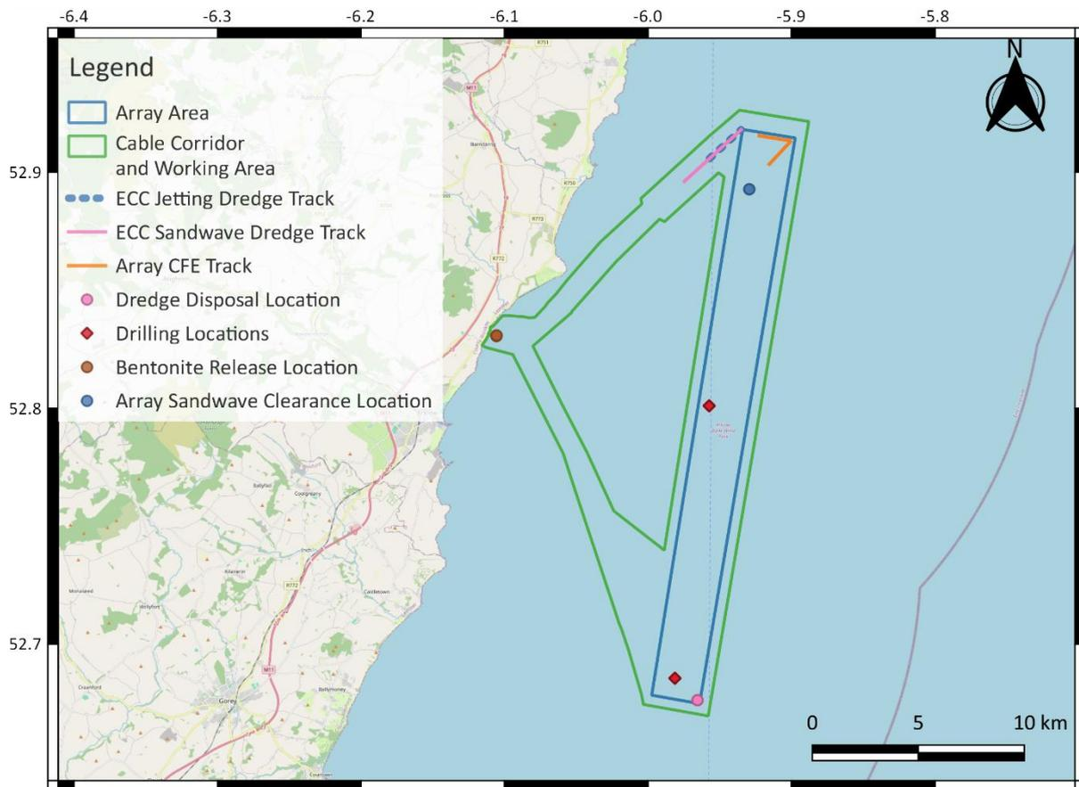
Figure 6.1.10: Locations used in particle tracking modelling.
